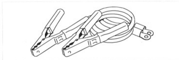
Figure 6 Cable for Direct Connection to 12 Volt Battery
